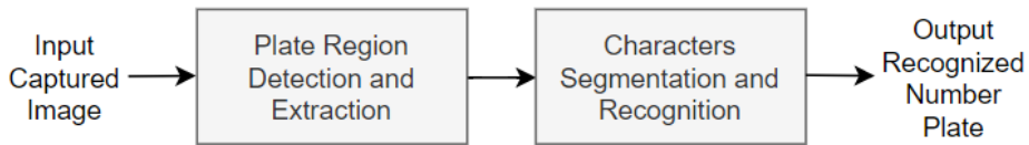
Fig. 1. Diagram of the ANPR system.
