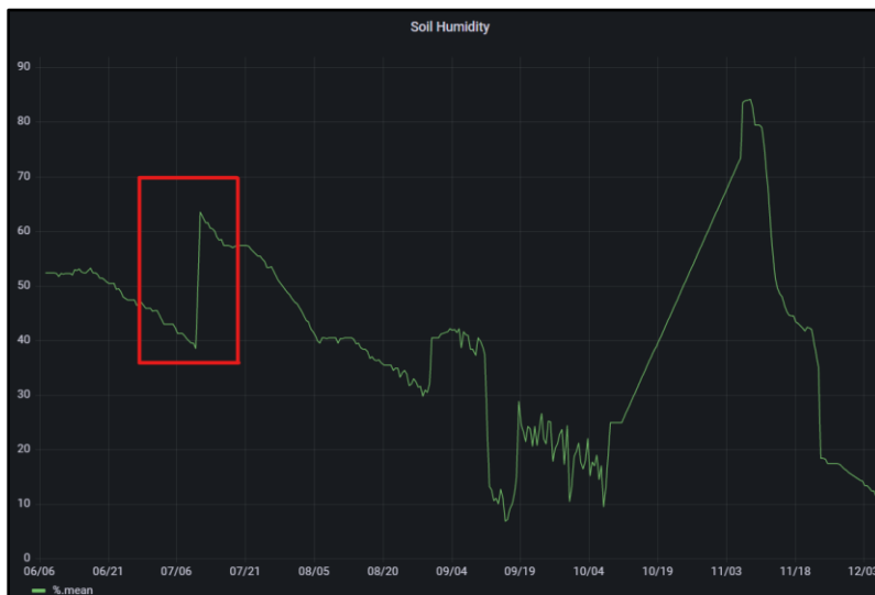
Fig. 6. Flooding incident as registered in Grafana Source: author's testing
